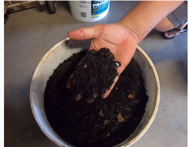
Activated carbon is a byproduct of TCOM
